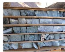
Figure 11.3.201 Core Processing. After Cut and Sampling Procedures
